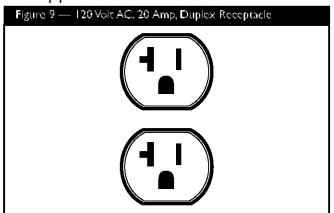
Use each receptacle to operate 120 Volt AC, single-phase, 60 Hz electrical loads requiring up to 2,400 watts (2.4 kW) at 20 Amps of current. Use cord sets that are rated for 125 Volt AC loads at 20 Amps (or greater).
